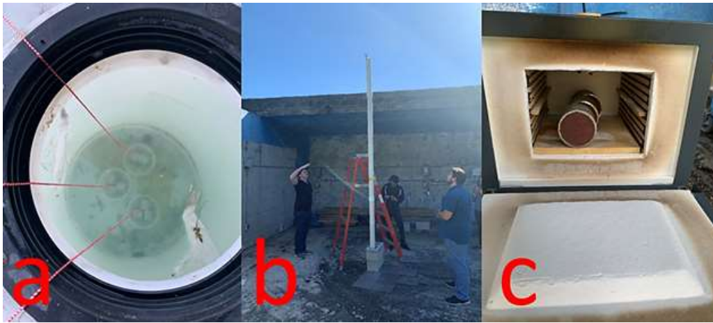
Figure 13. Experimental designs for relevant conditions testing. a) water testing b) drop/impact testing c) heat testing.
