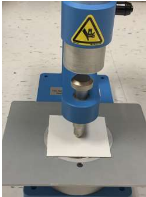
Figure 23. Illustration of coupon, coated side up, in test apparatus before impact.
